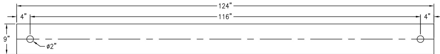
BASE PLATE ANCHOR HOLE DETAIL
