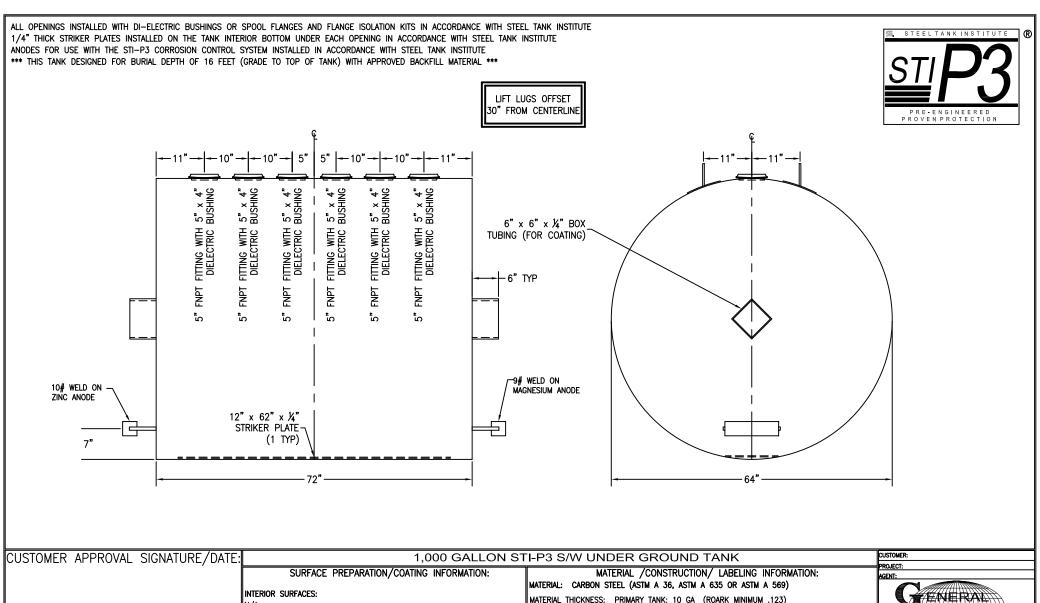
MATERIAL: CARBON STEEL (ASTM A 36, ASTM A 635 OR ASTM A 659)
