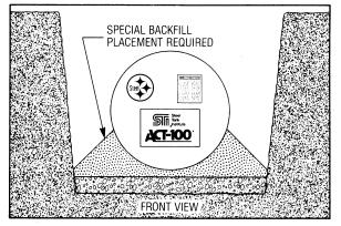
**6.2** Installing and tamping backfill along the bottom sides of the tank shall ensure that the tank is fully and evenly supported around the bottom quadrant.
