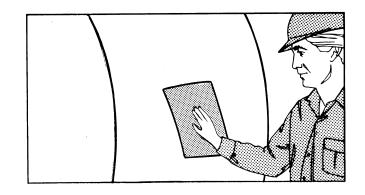
**3.2** Visually inspect the tank for damage. Pay particular attention to areas where laminate has been gouged or abraded. Mark all areas which appear damaged for repair. Any section of the laminate, which has been damaged beyond the surface of the laminate, shall be tested for holidays. This shall be done with a holiday detector set at a minimum 10,000 volts.
