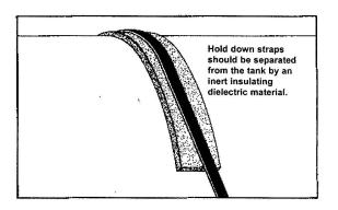
**5.2** If a metallic hold-down strap is used, a pad of inert insulating di-electric material must be used to insulate the hold-down strap from the tank. The separating pad shall be wider than the hold-sown straps, which will prevent direct
