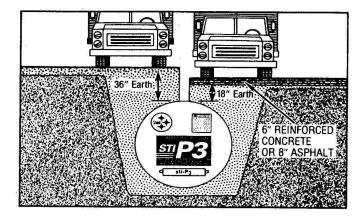
**11.1** Homogeneous backfill shall be deposited carefully around the tank and to a depth of at least one foot (305mm) over the tank. (See NFPA 30 and state or local codes for minimum depth of cover required).
