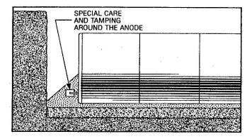
7.1 Homogeneous backfill similar to bedding material shall be placed carefully around the entire tank to create a uniform homogeneous environment. Avoid damage to coating especially where tamping is required.
