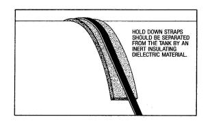
**6.2** If a metallic hold-down strap is used, a pad of inert insulating di-electric material must be used to insulate the hold-down strap from the tank. The separating pad shall be wider than the hold-sown straps, which will prevent direct contact between the straps and the tank shell. This pad is not
