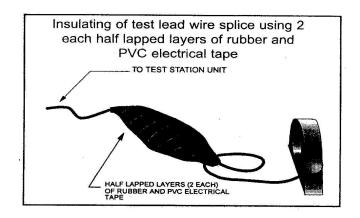
**9.6** Assure that the wire connection is strong by simultaneously placing tension on the wire at either side of the connection point. Protect the wire connection from corrosion using the material supplied with the PP4<sup>®</sup> or by wrapping the connection in half lapped layers of rubber and PVC electrical tape.
