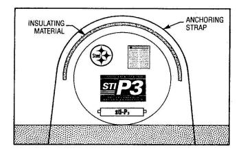
6.1 High water tables or partially flooded excavation sites exert significant buoyant forces on tanks. Buoyant forces are partially resisted by the weight of the tank, the backfill and the pavement atop the tank. Additional buoyant restraint, when required, shall be obtained by using properly designed hold-down straps in conjunction with concrete hold-down slabs or deadman anchors. The use of steel cable and/or round bar as hold-down straps on the tank is prohibited.
