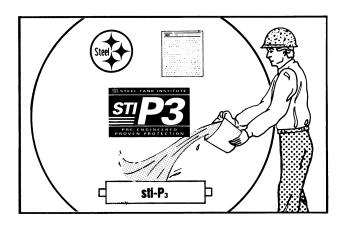
5.3 <u>To assure immediate operation of cathodic</u> protection system, each anode shall be thoroughly saturated with water at time of backfill operations.
