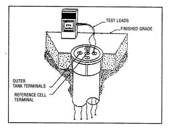
probes to the appropriate test head terminals as shown in the diagram above. As stated in 12.1, a minimum reading of -850 millivolts should be obtained.
