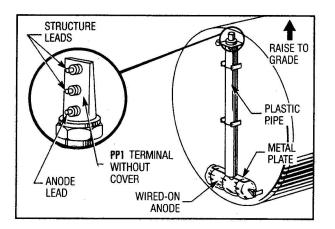
9.9 If the tank is equipped with a Protection Prover 1 (PP1<sup>®</sup>) monitoring system, which includes a monitoring test station mounted at the end of the tank, prior to any backfilling, extend the monitoring system to 4 inches (102 mm) below grade level without pulling it out of the mounting bracket. The PP1<sup>®</sup> test station shall be protected by a grade manhole of 7½ inches (191 mm) minimum diameter.
